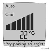
In AUTO mode the cooler will remember the last setting used. Press the button if you require more cool air or the button if you require less. Don't alter the setting however, until the room temperature has stabilised.
