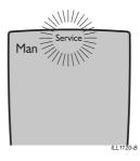
When "Service" is displayed it may be necessary for you to phone the service number located near the back of this manual. However, before doing so, turn the wall control OFF. You will notice a number flashing at the bottom of the screen. This number indicates the reason for requiring service.
