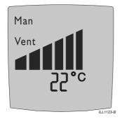
Once COOL or VENT has been selected, the wall control will maintain a constant fan speed. This is indicated by the bar graph shown on the display.
