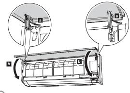
(4) Press 4 places on the intake grille to close it completely.
