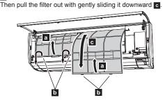
While holding the intake grille with your hand, pull up the handle
