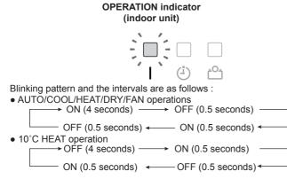
The indicator will keep blinking until the unit finishes the function.
