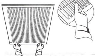
4. Slide the filter out from the core.
