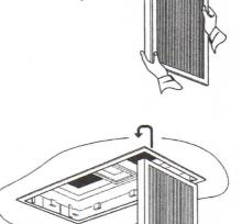
15. To ensure air flow through the filter is in the correct direction. Install the filter/s with the recess part of the filter facing down.
