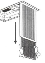
7. If a fresh air filter is fitted turn clips through 90° and remove filter.
